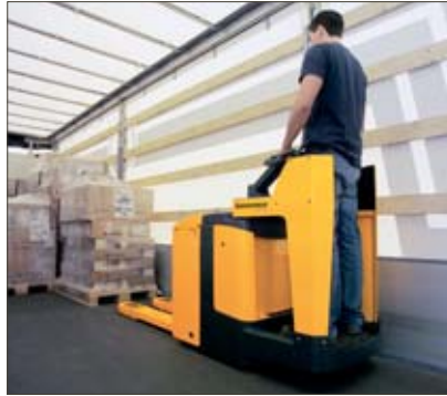
Protected operator workplace with fixed stand-on platform
